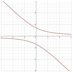
Clearly, there are tangent lines to this graph because everything looks smooth, but how do we find them? The trick to pretend that y is a function of x, (i.e. y = f(x)), then dy/dx will give us the slope of the tangent line at a point. Taking a derivative of both sides gives:
